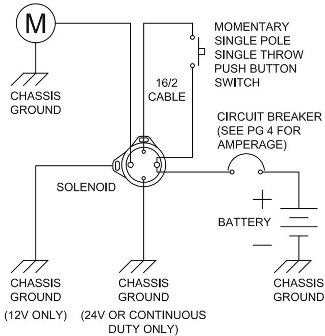
NOTE: SIZE CABLE PER AMPERAGE ON MOTOR NAME PLATE
