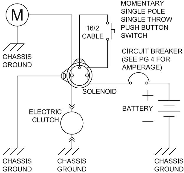
NOTE: SIZE CABLE PER AMPERAGE ON MOTOR NAME PLATE AND ADD 5 AMPS FOR ELECTRIC CLUTCH
