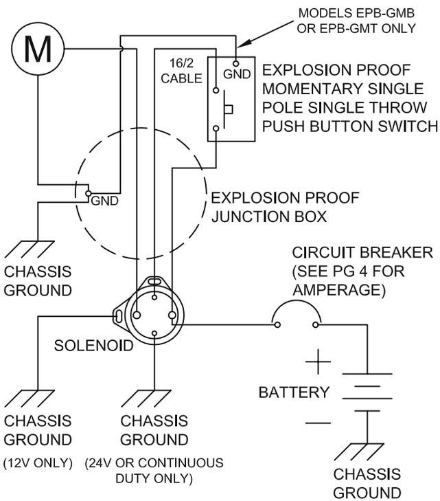
NOTE: SIZE CABLE PER AMPERAGE ON MOTOR NAME PLATE
